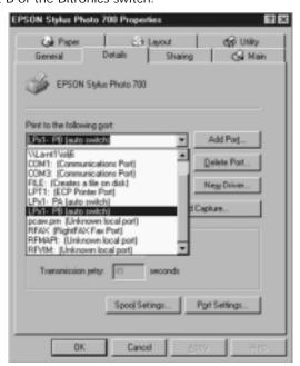
In the image above, the printer is connected to Port B of the Bitronics switch. Therefore, LPx1 – PB (autoswitch) is selected. When finished, click OK.
